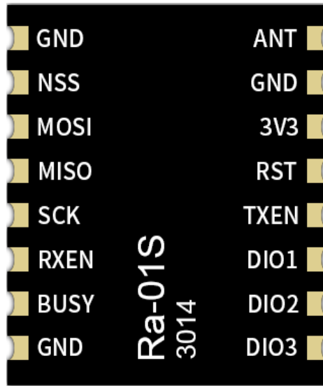
Ra-01SC Pin diagram
