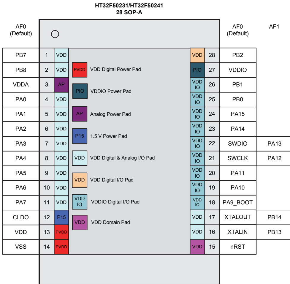
Figure 6. 28-pin SOP Pin Assignment
