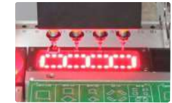
To improve the machine adaptability,it is adopted 4 head synchronous identification and mounting solution.
