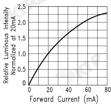
Fig.4 Relative Luminous Intensity
