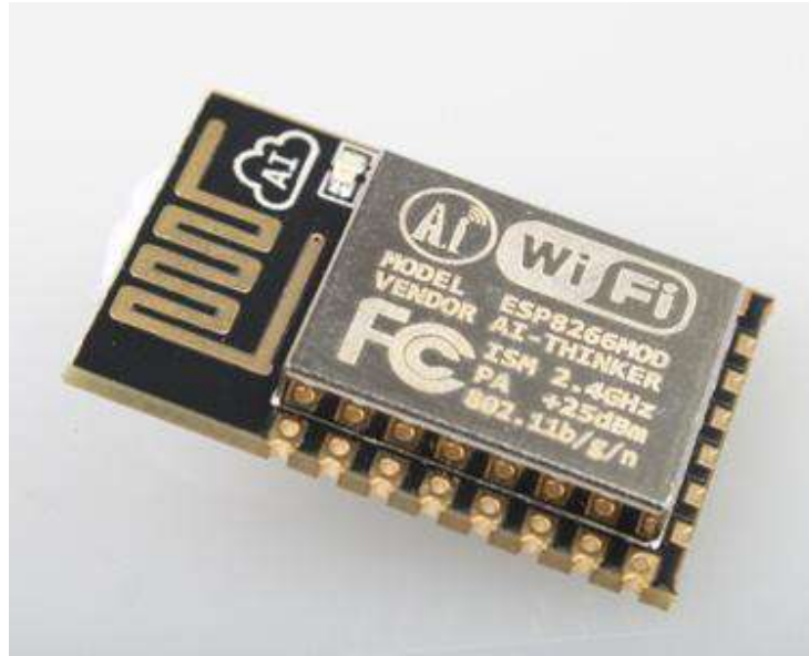
Figure 3 [Module Pin Counts, 22 pin, 16 mm *24 mm *3 mm]
