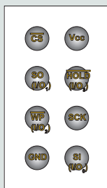
Figure 1-3. 8-ball WLCSP (Bottom View)
