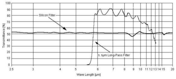
Note: The graph shows a typical 5um infrared filter reference, and the curve is the average of infrared pass rate. The window material is a special vacuum coating of semiconductor wafers.
