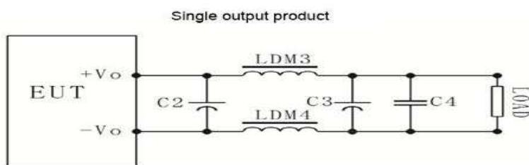
When the requirements on ripple & noise are normal, it is recommended to use only C2 in the periphery; when the requirements on ripple & noise are strict; the circuit above is recommended.
