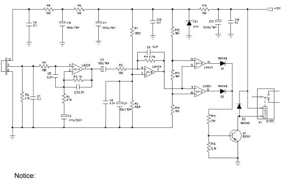
U1A-D:LM324 Vdd:12V DC Rs=47KΩ @ on an offset voltage
