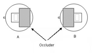
The sensitivity balance of sensor is calculated by measuring the sensitivity (signal output voltage) of each side and uses the formula as below:
