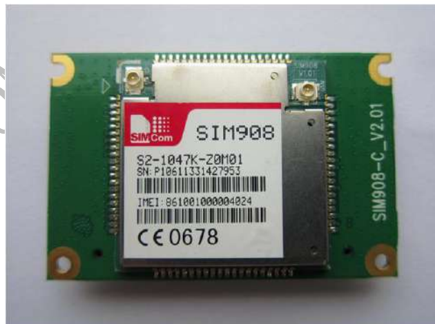
Figure 41: Top view of SIM908-C
