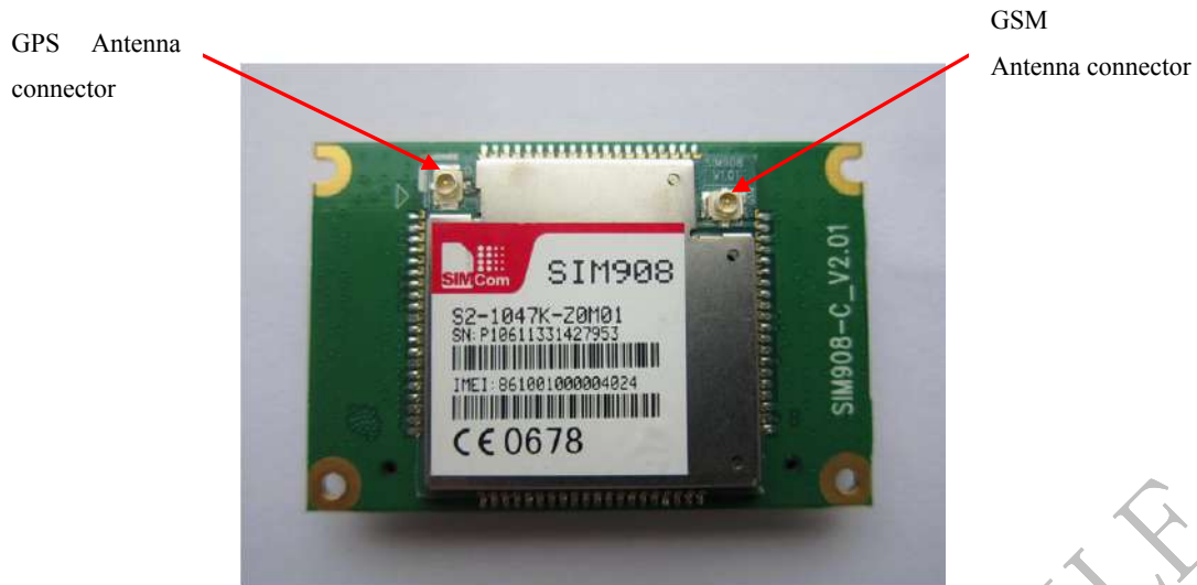
Figure 38: The RF interface of module
