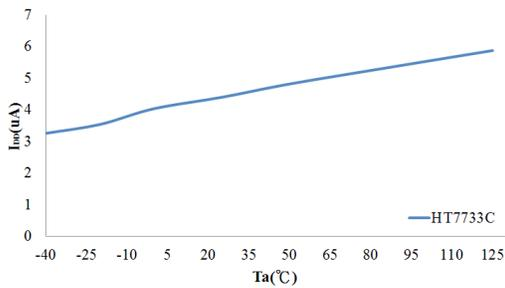
**HT7733C I<sub>DD</sub> vs. Ta**
