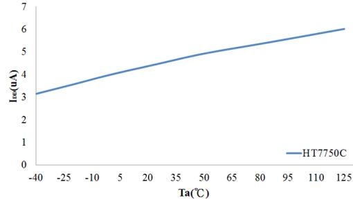
**HT7750C I<sub>DD</sub> vs. Ta**
