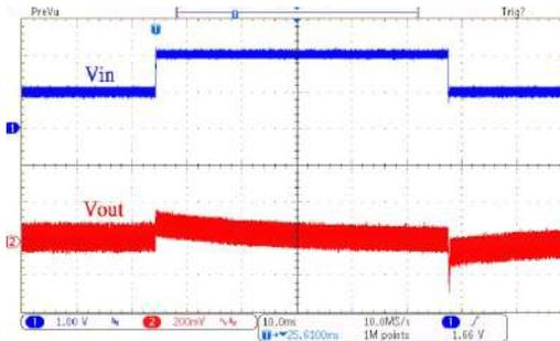
**HT7733C Line Transient (1V to 2V,  $I_{OUT}=50mA$ )**
