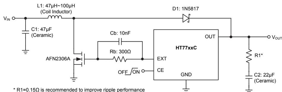
Note: 1. When CE='0', the device internal circuits such as the bandgap reference, gain block and all feedback and control circuitry will be switched off.
