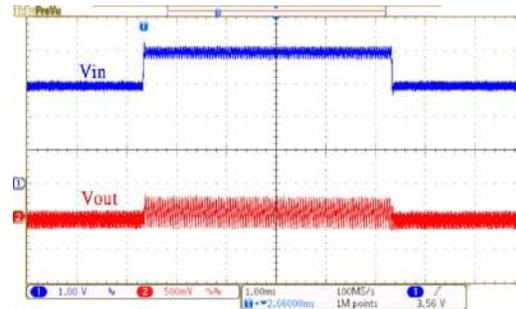
**HT7750C Line Transient (3V to 4V,  $I_{OUT}=100mA$ )**
