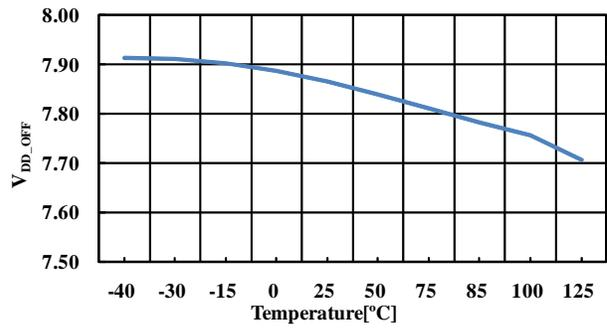
Figure 14. V<sub>DD\_OFF</sub> vs. Temperature
