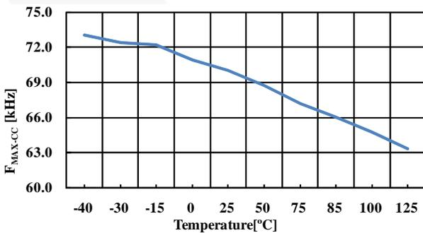
Figure 17. f<sub>MAX\_CC</sub> vs. Temperature
