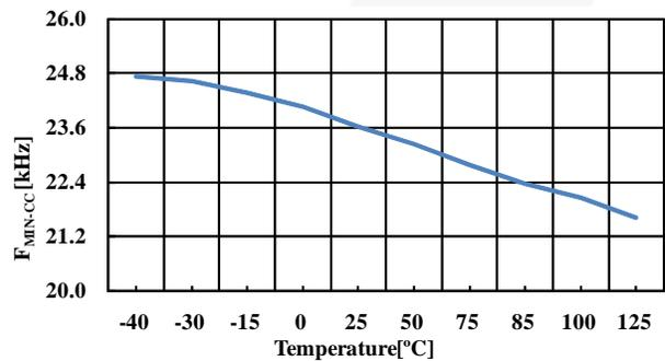
Figure 18. f<sub>MIN\_CC</sub> vs. Temperature
