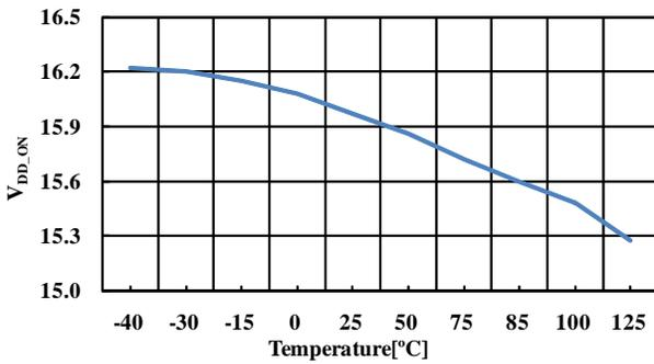
Figure 13. V<sub>DD\_ON</sub> vs. Temperature
