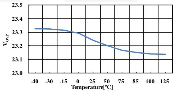
Figure 16. V<sub>OVP</sub> vs. Temperature
