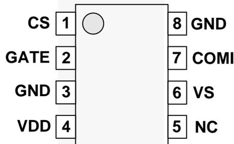
Figure 4. Pin Configuration
