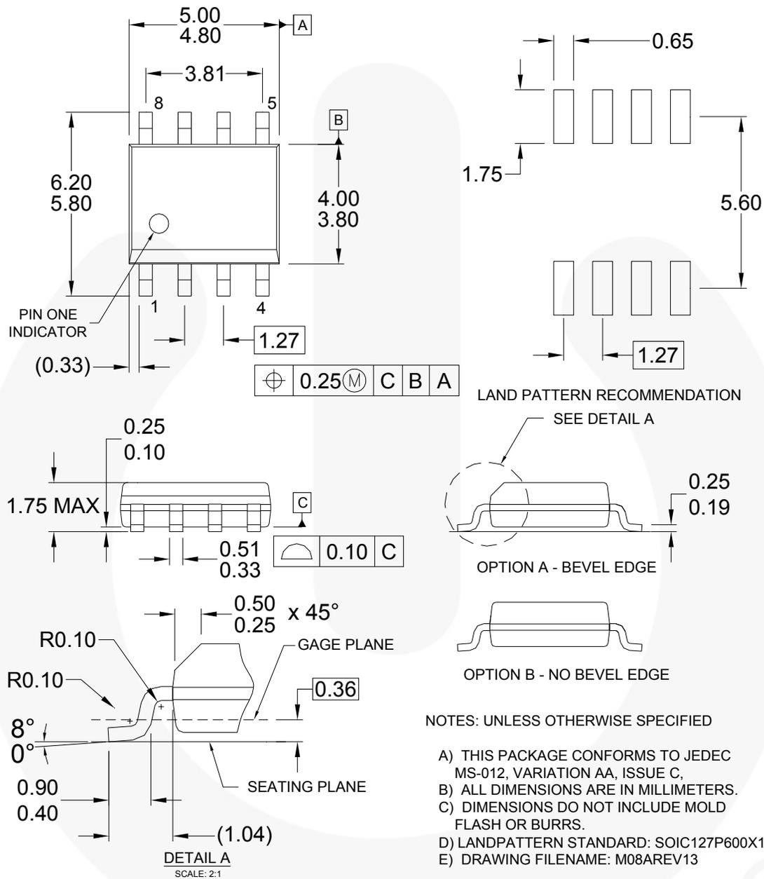
Figure 23. 8-Lead, Small Outline Integrated Circuit Package (SOIC)
