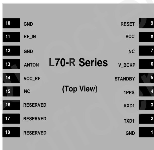
Figure 2: Pin Assignment
