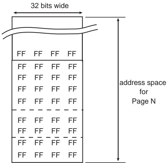
Step 1: Flash array after page erase
