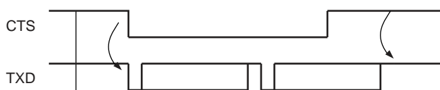
Figure 36-28. Transmitter Behavior when Operating with Hardware Handshaking
