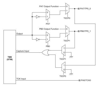
TM0 Function Pin Control Block Diagram
