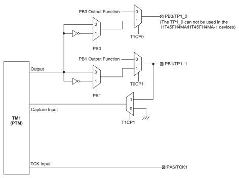
TM1 Function Pin Control Block Diagram
