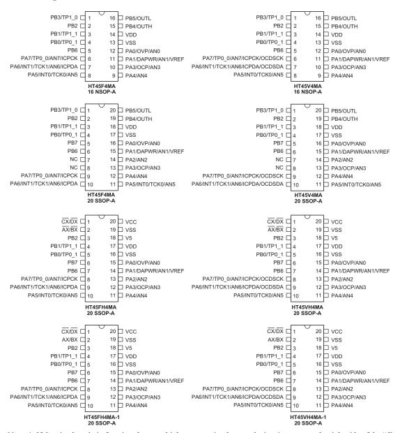
Note: 1. If the pin-shared pin functions have multiple outputs simultaneously, its pin names at the right side of the "/" sign can be used for higher priority.
