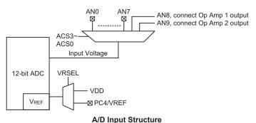
The A/D converter has its own reference voltage pin, VREF, however the reference voltage can also be supplied from the power supply pin, a choice which is made through the VRSEL bit in the ACSR register. The analog input values must not be allowed to exceed the value of VREF.
