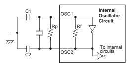
Note: 1. Rp is normally not required. C1 and C2 are required.2. Although not shown OSC1/OSC2 pins have a parasitic capacitance of around 7pF.
