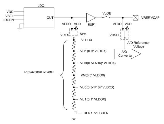
Note: 1. The total resistance of the divided resistors can be  $500k\Omega$  or  $200k\Omega$  selected using the ISEL bit in the LCDC register.
