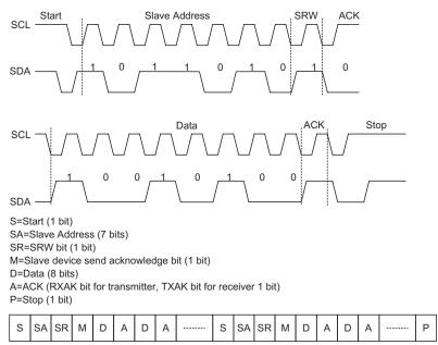
Note: \* When a slave address is matched, the device must be placed in either the transmit mode and then write data to the SIMD register, or in the receive mode where it must implement a dummy read from the SIMD register to release the SCL line.
