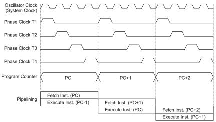
System Clocking and Pipelining
