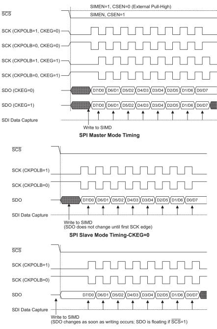
Note: For SPI slave mode, if SIMEN=1 and CSEN=0, SPI is always enabled and ignores the  $\overline{SCS}$  level.
