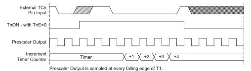
Pulse Width Capture Mode Timing Chart (TnE=0)
