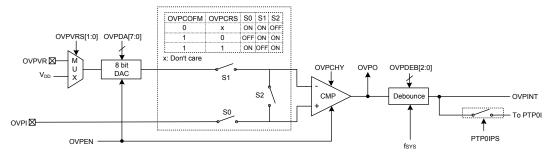
**Over Voltage Protection Circuit**
