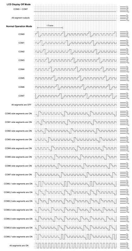
LCD Driver Output - Type A, 1/8 Duty, 1/3 Bias
