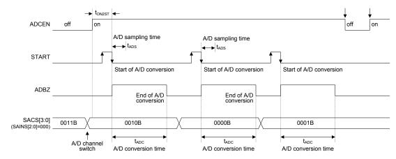
A/D Conversion Timing – External Channel Input
