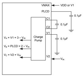
Power Supply from pin V2
