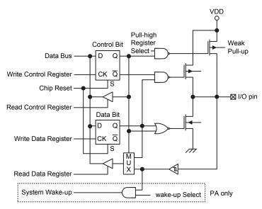
**Logic Function Input/Output Structure**
