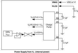
Note: The pin VMAX must connect to the maximum voltage to prevent from the pad leakage.
