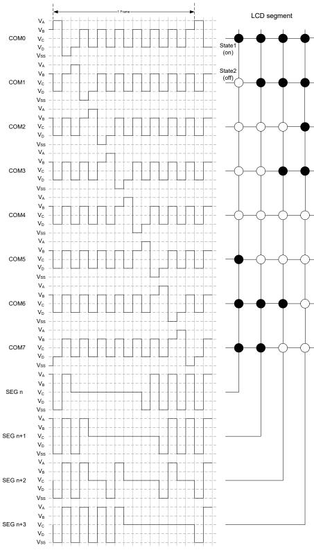
LCD Driver Output - Type A, 1/8 Duty, 1/4 Bias
