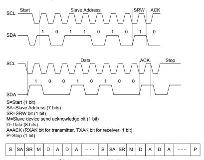
I<sup>2</sup>C Communication Timing Diagram
