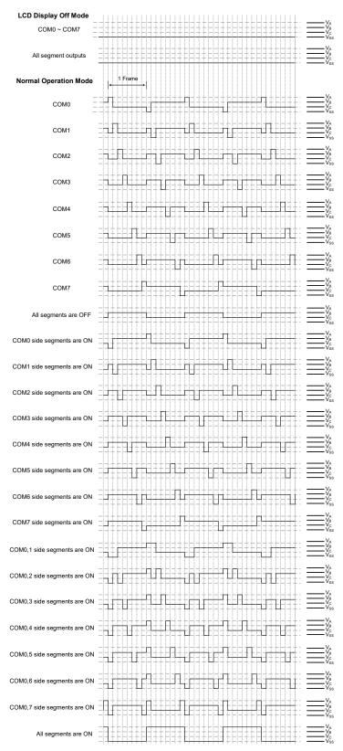
LCD Driver Output - Type B, 1/8 Duty, 1/3 Bias
