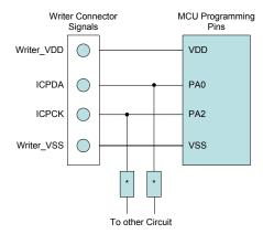
Note: \* may be resistor or capacitor. The resistance of \* must be greater than  $1k\Omega$  or the capacitance of \* must be less than 1nF.
