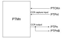
PTM Function Pin Control Block Diagram - n=0~2
