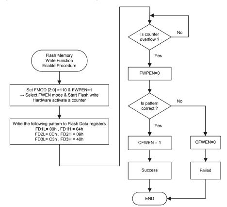
Flash ROM Write Function Enable Procedure
