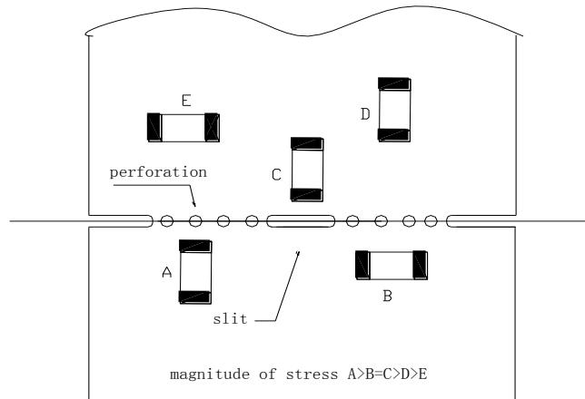
When breaking PC boards along their perforations, the amount of mechanical stress on the capacitors can vary according to the method used. The following methods are listed in order from least stressful to most stressful: push-back, silt, -grooving, and perforation. Thus, any ideal SMD capacitor layout must also consider the PCB splitting procedure.
