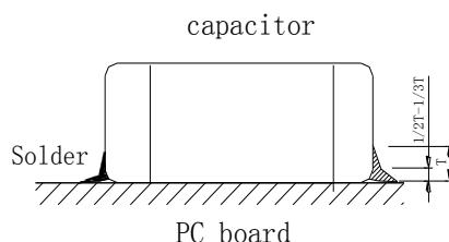
②. Because excessive dwell times can detrimentally affect solderability, soldering duration should be kept as close to recommended times as possible.
