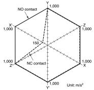
Sample: G2RL-24 12 VDC Number of Relays: 5 pcs Test conditions: Shock is applied
