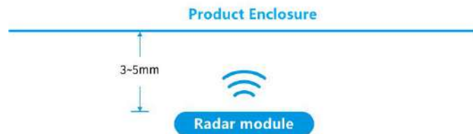
Figure 3 The distance between the antenna surface and the product shell
